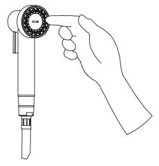
Any deposits which may accumulate on the nozzle can be removed by simply running a finger over the rubber extrusions and then running the water for a few seconds. In extreme cases this step may have to be repeated.
